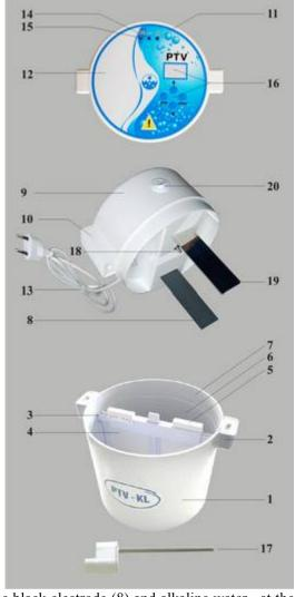
4.5. During water electrolysis acidic water is generated at the black electrode (8) and alkaline water - at the light one (19). Partition (4) of the removable vessel (3) doesn't allow ionized water to mix.
